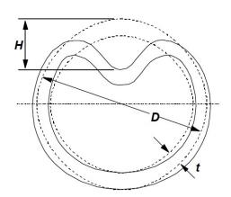
$$\begin{split} N_c &= 562.2 \left[ \frac{\sigma_{uts}}{2\sigma_A K_d K_g} \right]^{5.26} \\ \sigma_A &= \sigma_a \left[ 1 - \left( \frac{\sigma^C_{m,max} - \sigma_a}{\sigma_{uts}} \right)^2 \right]^{-1} \\ \sigma_a &= \frac{\sigma^C_{m,max} - \sigma^C_{m,min}}{2} \\ K_d &= 1 + C_s \sqrt{\frac{t_c}{D_o} \left( d_{d0} \cdot C_{ul} \right)^{1.5}} \\ C_s &= 2.0 & (for smooth dents, r_d \ge 5t_c) \\ C_s &= 1.0 & (for sharp dents, r_d < 5t_c) \\ K_g &= 1 + 9 \left( \frac{d_g}{t} \right) \end{split}$$
